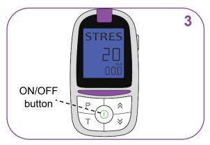
Press and hold the ON/OFF button to switch the device on
